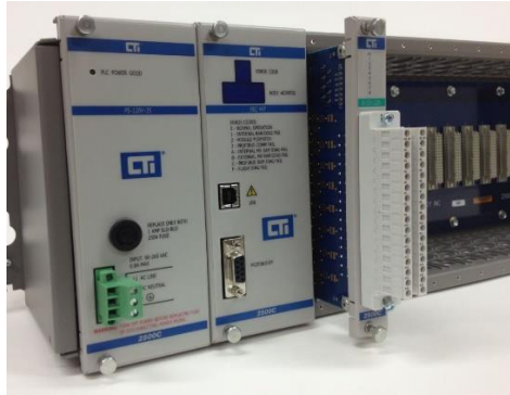
Figure 28 2500C-8-TC Module Physical Installation Picture
