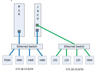
Port A is connected to a plant "data" network, used for programming and data access (HMI and SCADA workstations). Devices on this network are members of the IP subnet 172.18.12.0/24 (172.18.12.1, 172.18.12.2, etc.).
