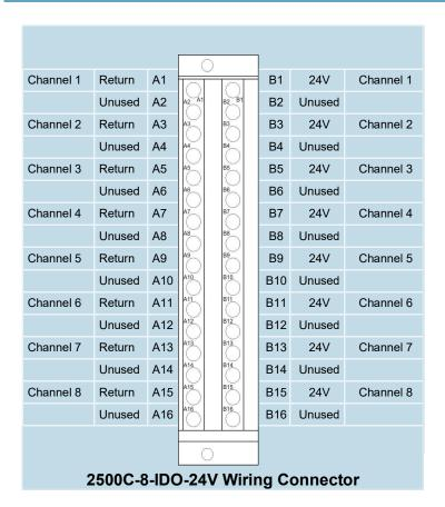
The 2500C-8-DO-24V Discrete Output Modules use CTI Wiring Connector 2500C-32F. Please see the wiring connector specification table below. This connector is ordered separately from the module.
