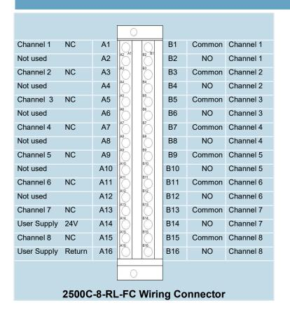
Note: The 2500C-8-RL-FC Relay Output Module uses CTI Wiring Connector 2500C-32F. Please see the wiring connector specification table below. This connector is ordered separately from the module.
